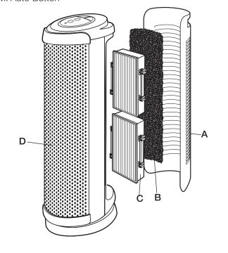
The filter may appear discolored, even after vacuuming. This is normal and does not affect performance in any way—a new filter is not necessary.
